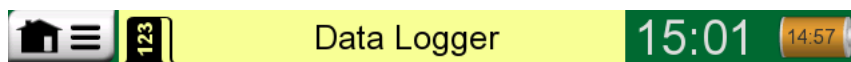
Figure 106: Title bar's active area (shown as yellow) for toggling between main view and graph view
